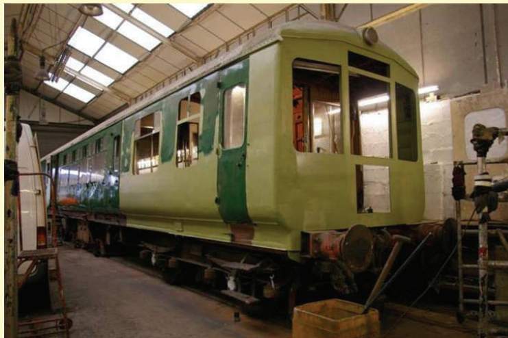
56097, body repairs to the first class saloon now completed (Llangollen Railcar Group)
