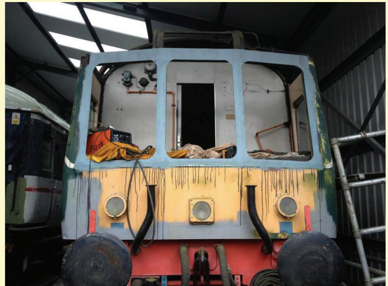
M55006, cab roof dome off and metalwork repairs progressing in January (L. Gratton)
